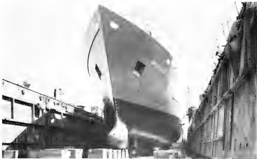
R/V Melville (AGOR 14) in drydock – shown are the underwater bow observation chamber and forward cycloidal propeller.
