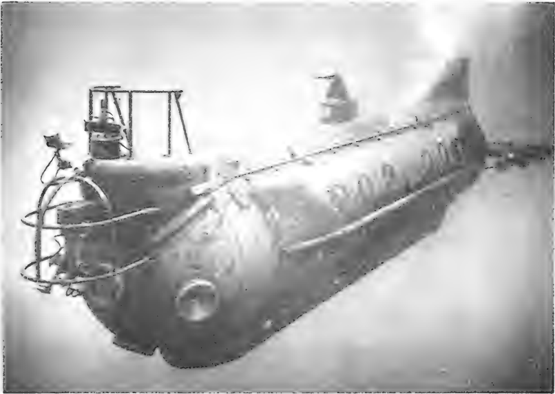
ALUMINAUT , a research vessel uniquely constructed of aluminum rings, for operation to depths of 15,000 feet.
