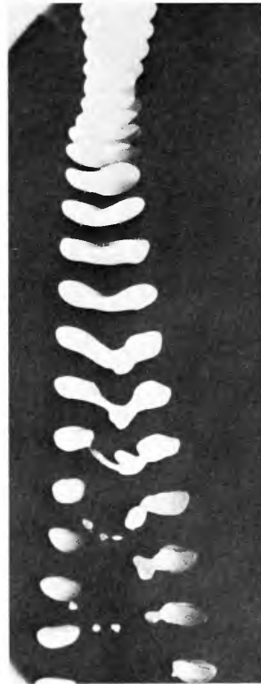
Laboratory photograph of raindrop disintegrating in upward moving airstream.
