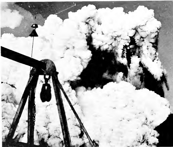
The antenna used to measure the atmospheric potential gradient on the chartered fishing boat 'Haraldur'.
