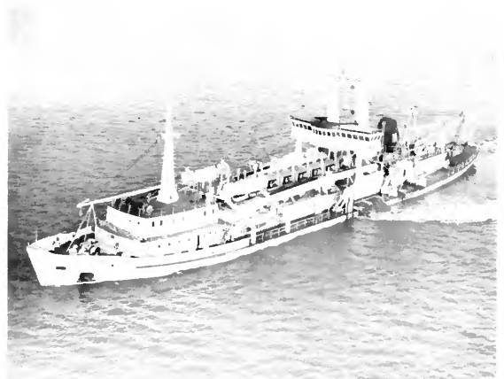
Figure 5. Trailing suction hopper dredge Yolanda underway while dredging sand and gravel in the North Sea. The vessel is almost fully loaded. (Skyfotos, Hythe, England)
