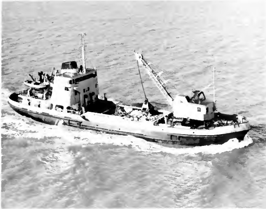
Figure 6. Ocean-going clamshell, or grab bucket, dredge Landguard at work in U.K. waters. This type is used mostly for harbor clearance but also may dig for gravel. (Skyfotos, Hythe, England)
