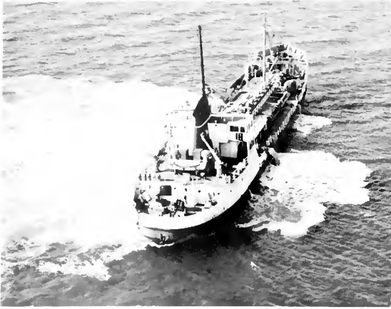
Figure 4. Suction hopper dredge Cambrook working in a stationary mode in the River Thames estuary. Over 2000 tons capacity, the vessel is one of the largest of the U.K. fleet. (Skyfotos, Hythe, England)
