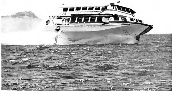
High-speed passenger transit is provided by the Boeing Jetfoil 929 hydrofoil, this one on SeaFlite service in Hawaii. The craft can carry as many as 250 passengers through high seas at almost 45 knots. Such forms of marine transportation will facilitate the evolution of floating platform communities. (Boeing Aerospace Company)
