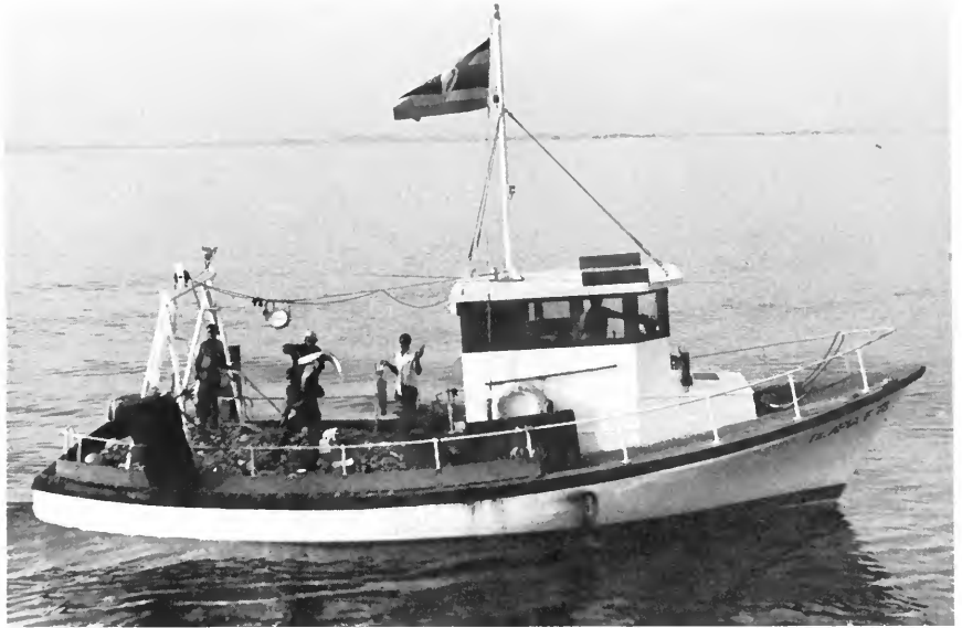
Figure 6. A ferro-cement trawler on Lake Victoria, East Africa. The vessel was built as a prototype and operated by the Food and Agriculture Organization of the United Nations under technical assistance projects. (Photo by author)
