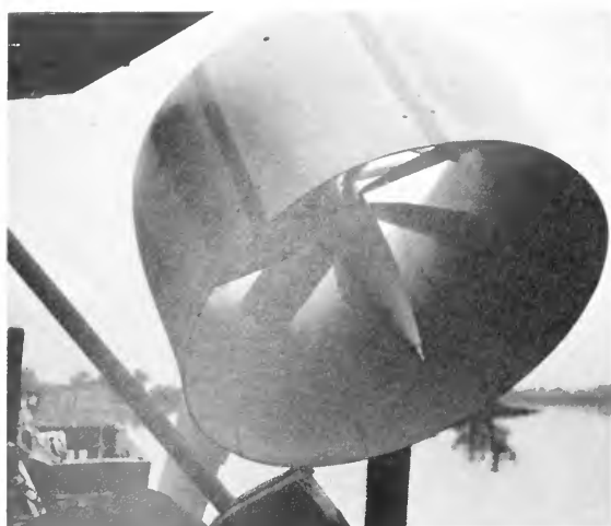
Figure 1. Rotor/duct unit (1.5 meters) undergoing testing.
