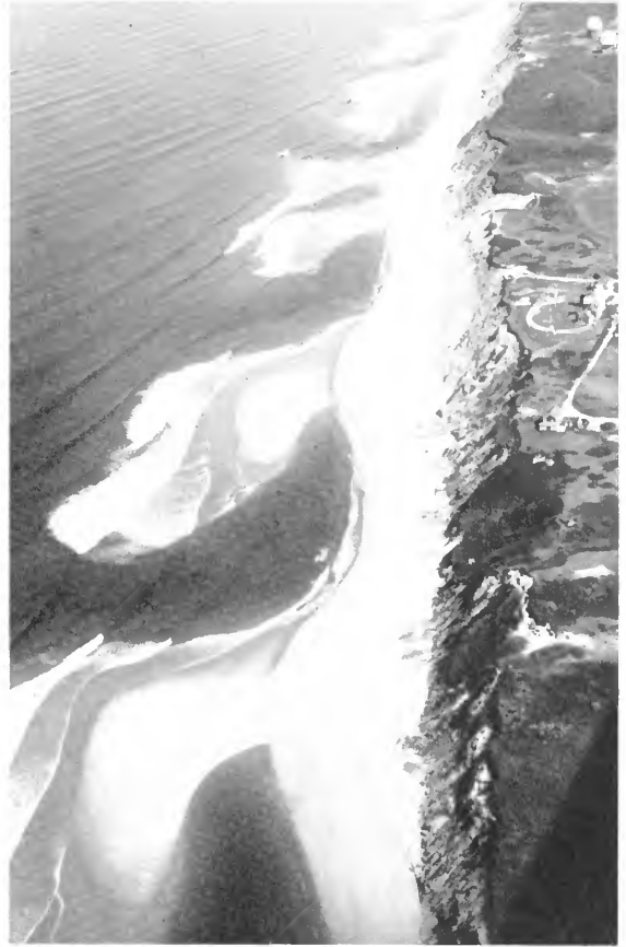
Figure 11. Multiple, shore-attached hooked bars stretching from Provincetown, to points further south along the Atlantic shore of Cape Cod, Massachusetts. The hooks point in the direction of longshore transport, and occur with a spacing of hundreds of meters.
