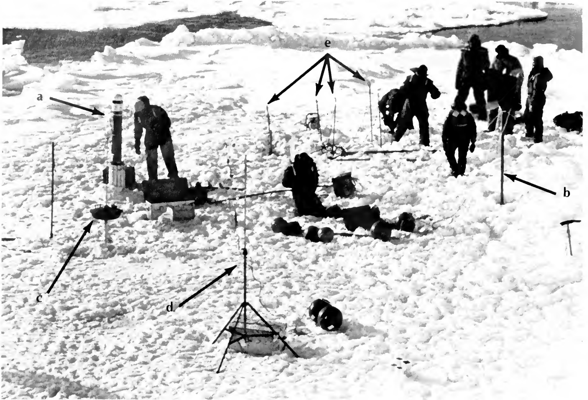
This ice floe in the Bering Sea marginal ice zone was instrumented to measure ablation, or melting, of the ice and illustrates most of the remote instrumentation that was used on the ice during MIZEX West. A radar transponder (a) and reflector (difficult to discern against the people in the background) atop a pole (b) allow the floe to be continually tracked by the ship. A wave disc buoy (c) contains an accelerometer that measures wave-induced ice motion; these data are then telemetered to a receiver on the ship. An internally recording anemometer (d) measures winds over the floe. The vertical staffs (e) are instruments designed to measure vertical melting rate. Not shown is a current meter that was suspended beneath the floe to measure relative ice/water motion. The numerous spheres are flotation devices that are attached to the instruments in case the floe breaks up before the ship can retrieve the gear. (Photo by author)
