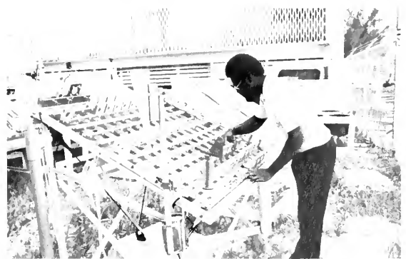
An ocean engineer on the campus of the University of Miami's Rosenstiel School of Marine and Atmospheric Science checks samples of various metal alloys for evidence of corrosion. (Photo by John Park, University of Miami)
