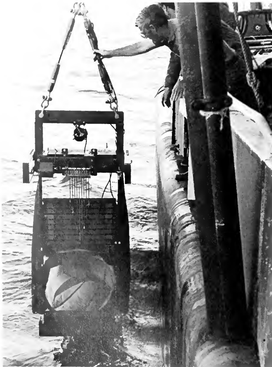
The 9-net MOCNESS-1/4, entering the water for a 0-to-200-meter oblique tow in a warm-core ring. (Photo by Peter Wiebe)
