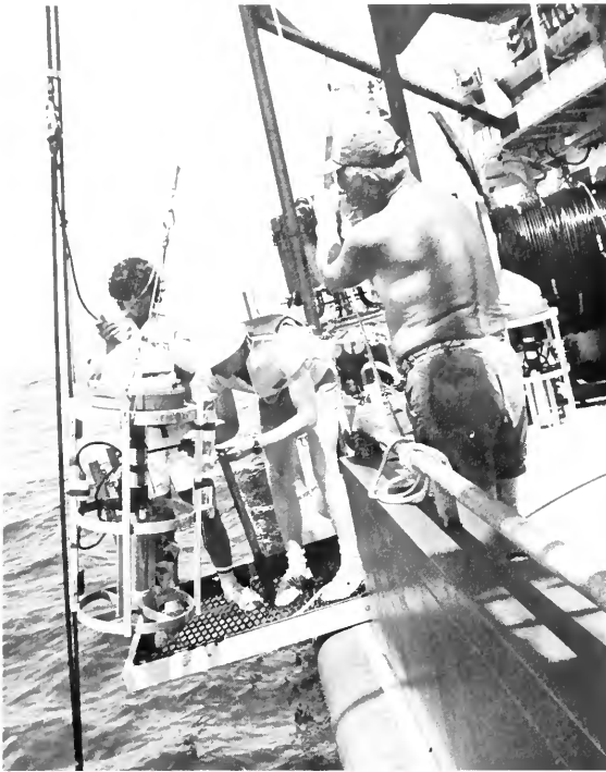
A unit of MULVFS (Multiple Unit Large Volume Filtering System) being attached to a conducting and support cable aboard the Oceanus . (Photo by Peter Wiebe)
