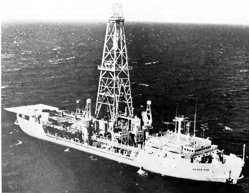
The Sedco 445, among the most experienced deep-water drillships in the world. (Courtesy of Sedco)
