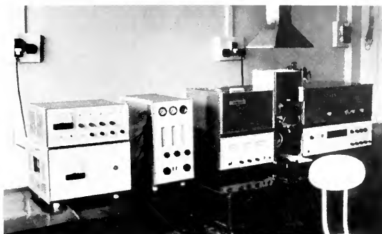
Atomic absorption spectrophotometer at the South China Sea Subbureau in Guangzhou. This Chinese-built double beam instrument with background correction was not yet in use at the time of the delegation's visit. (Courtesy of authors)
