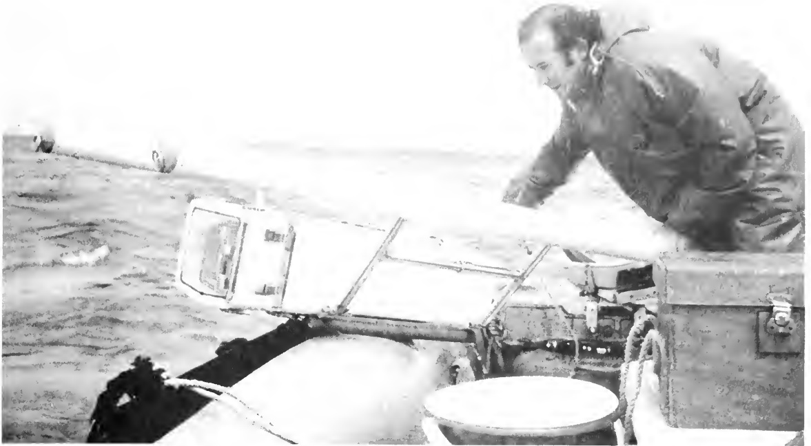
Figure 1. A floating instrument package capable of providing sophisticated, high-resolution measurements of reef flat productivity and calcification. (a) The instrument package is deployed from a small, inflatable boat moored in shallow water on a reef flat. (b) The package floats across the reef flat with the current and records changes in seawater pH, oxygen content, and temperature, as well as the incident light intensity. (Photo courtesy of the authors)
