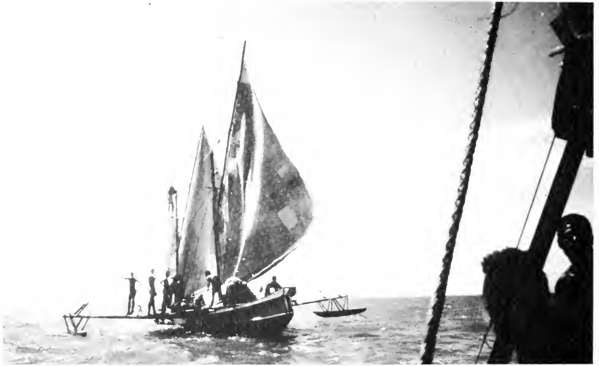
A double-outrigger canoe under sail. When these larger canoes were developed in the 1920s, they extended the range and time on the reef of the Kiwai hunters. (Photo courtesy of John Mason)
