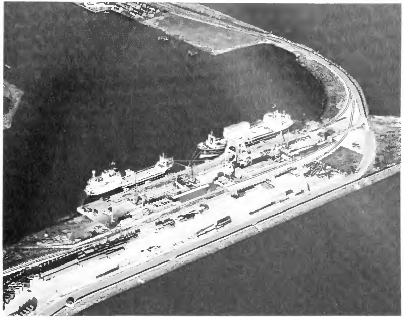
Figure 3. Reprocessing fuel from overseas involves sea transport of spent nuclear fuel. Several purpose-built ships owned by BNFL's subsidiary, Pacific Nuclear Transport Limited, or by BNFL itself, are used. The larger ships each have a capacity of 28 flasks and a total load of 60 tons of spent fuel. The fuel flasks are offloaded at the BNFL terminal at Barrow. (Courtesy BNFL)
