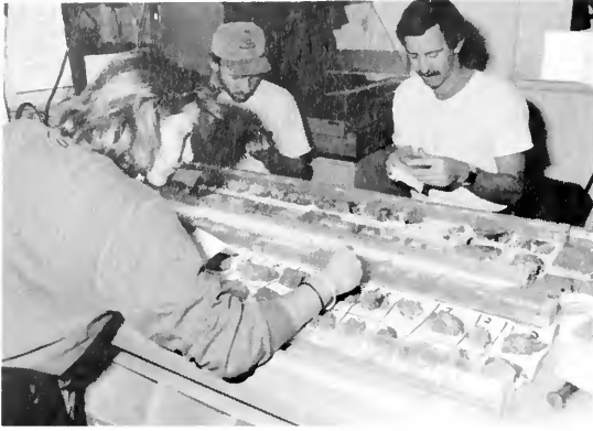
Marine technicians Henrike Groschel, Greg Simmons, and Harry (Skip) Hutton number and label pieces of basalt recovered from the Mediterranean on Leg 107.
