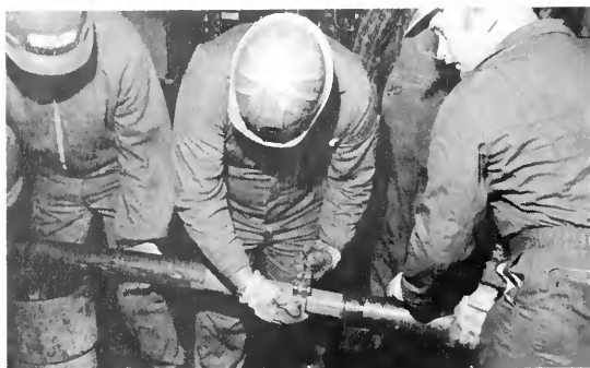
On the rig floor, the crew removes the 31-foot-long (9.5 meters) core from the core barrel. It is cut into 5-foot sections for analyses.
