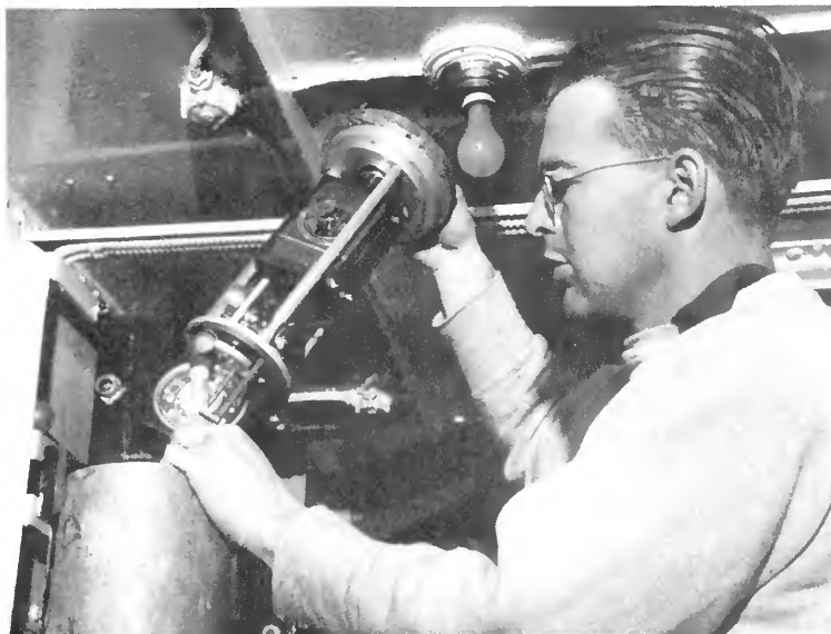
Preparing to test, in 1940, the first remotely controlled camera that could photograph the deep ocean floor. (WHOI Archives)
