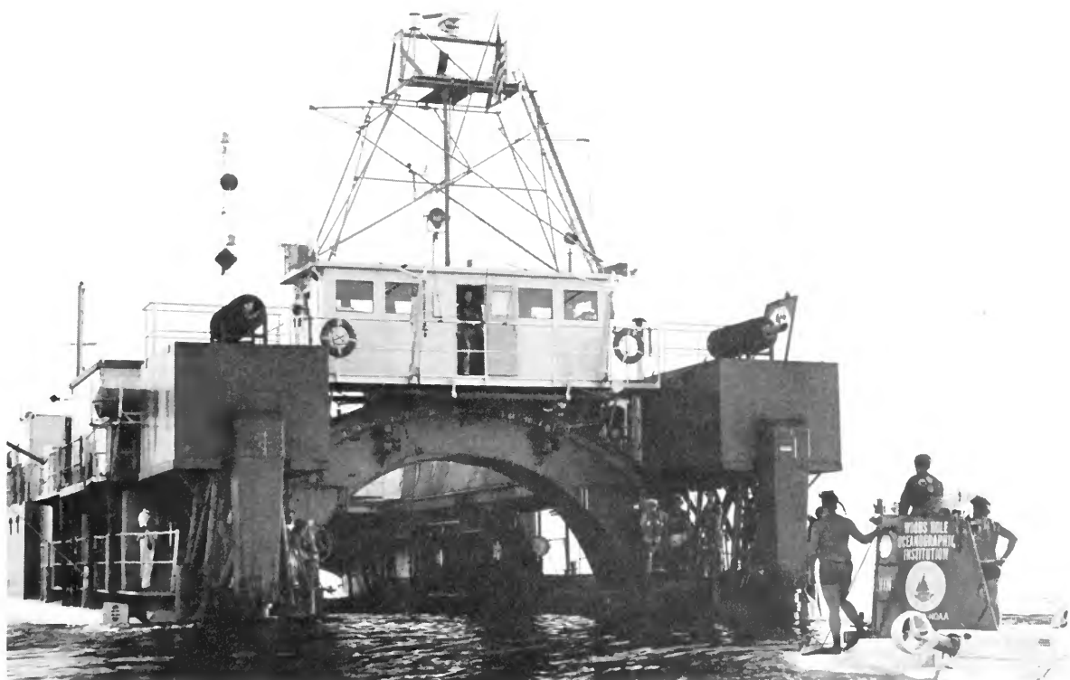
Lulu awaits the return of Alvin at the end of a dive. Lulu served as the mother ship until R/V Atlantis II was modified to perform this function in 1983. (Photo courtesy of WHOI)
