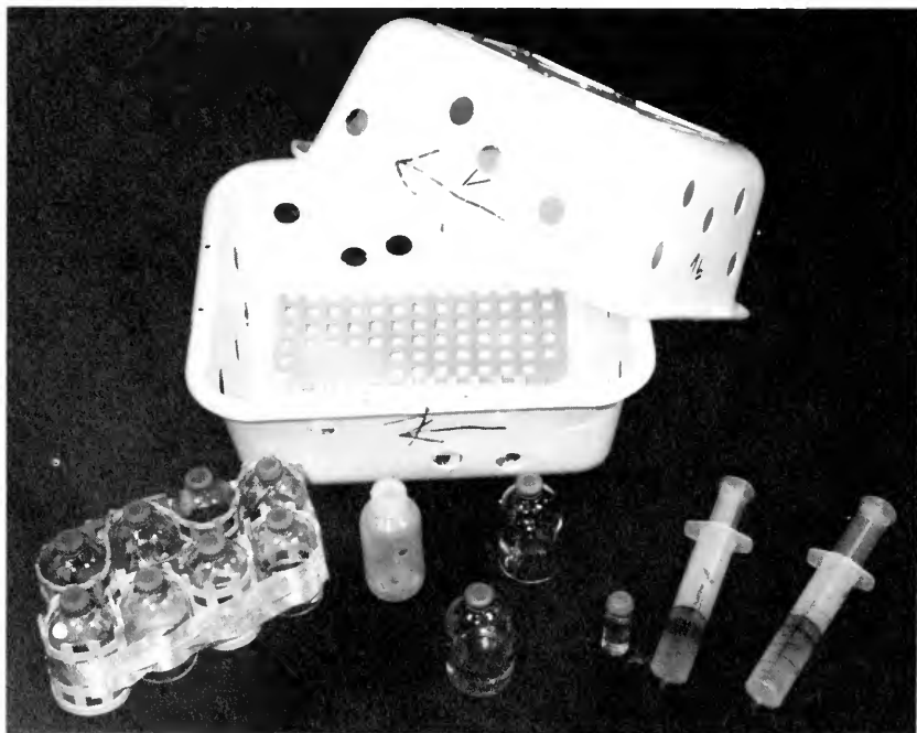
Figure 1. The equipment used in the first controlled repeat of Alvin's unintentional venture into microbiology. The boxes, made from plastic household dish pans, held a variety of sample vessels. The boxes were fastened to the mooring chain of deep-sea buoys, and incubated for 5 months.
