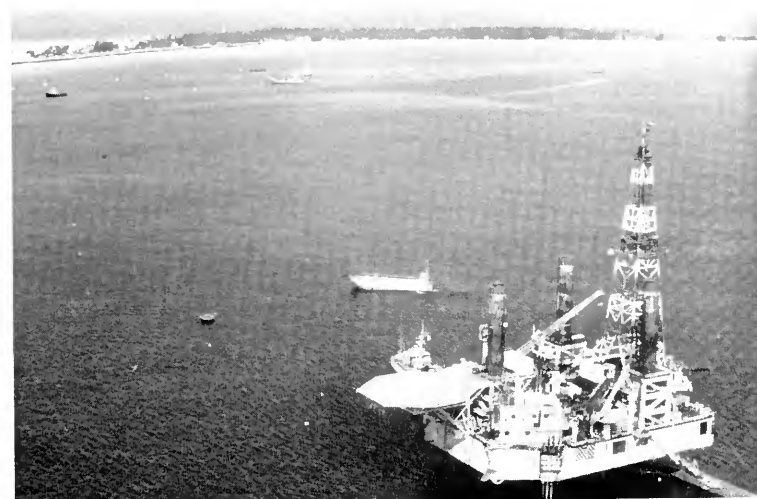
At top, an aerial view of Mururoa in French Polynesia, where (middle) the French prepare a site for nuclear-weapons testing. At bottom, drilling rigs in the lagoon bore holes as much as 1,000 meters deep for nuclear tests. (Top, photo by Jean Gaumy/Magnum; middle, Robine/Agence France-Presse; bottom, Herrmann/Sipa Press)
