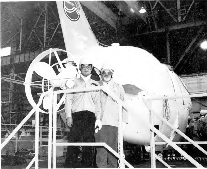
The author and Japanese colleague finish inspecting a new manned submersible, the Shinkai-6500, at Mitsubishi's Kobe plant. The submersible is the deepest-diving manned vehicle in the world, capable of working at 6,500 meters, giving it access to 98 percent of the world's seafloor. (Courtesy of author)
