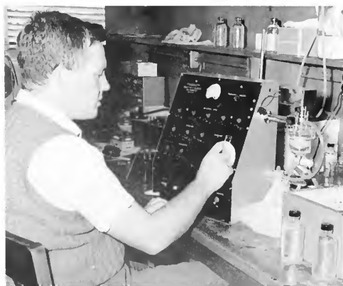
In this 1960 photograph, the author operates an early inductively coupled salinometer.
