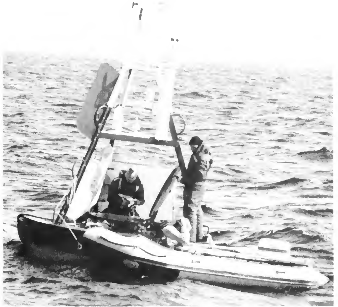
The R-TEAM surface module has an umbilical attached to a subsurface flotation module 100 meters below the surface.
