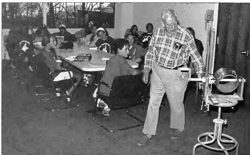
Using the Compton generator, Hank Stommel demonstrates the Coriolis force for a junior high school class in 1991.
