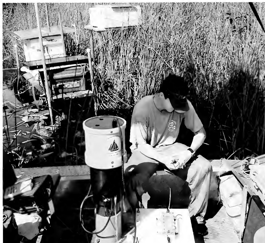
AUTOMATED MEASUREMENTS —Research Assistant Matt Allen sits on an airboat and sets up a WHOI-designed automated seepage meter for a three-week deployment in Florida's Everglades.
