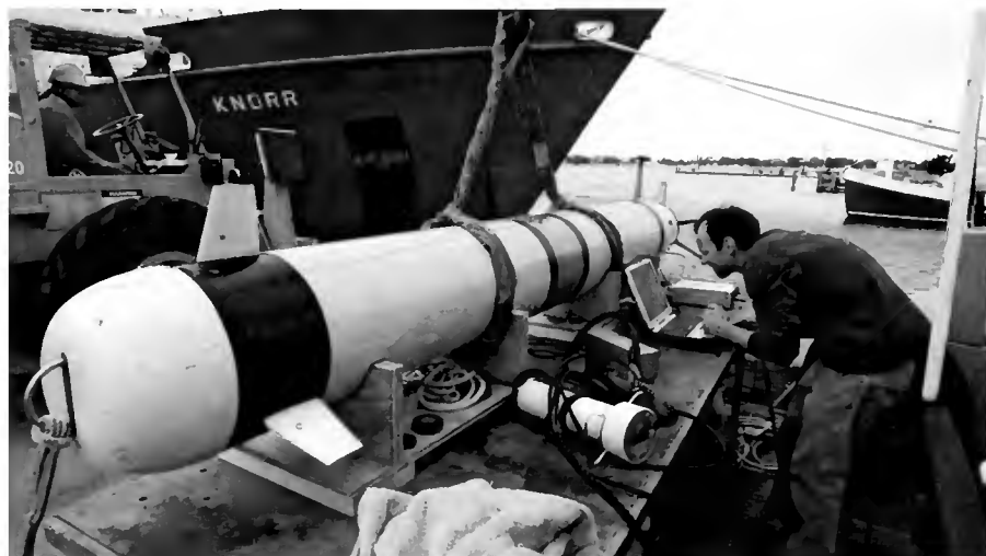
UNDERWATER RECONNAISSANCE—WHOI Senior Engineering Assistant Greg Packard puts a REMUS 600 autonomous underwater vehicle through a series of pre-launch checks on the WHOI dock before it is tested in the waters near Woods Hole. Crane operator Doug Handy stands by. The REMUS 600 can carry a variety of sensors for underwater surveying and mapping and, not incidentally, can be deployed through submarine torpedo tubes.
