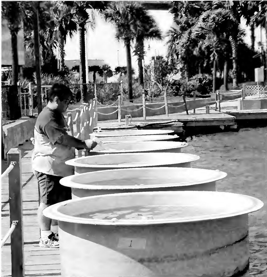
TEXAS TWO-STEP —In an experiment in Corpus Christi, Texas, WHOI scientist Mario Sengco pumped algae-rich water into tanks and treated them with clay. Within hours, the sinking clay removed more than 70 percent of the algae.
