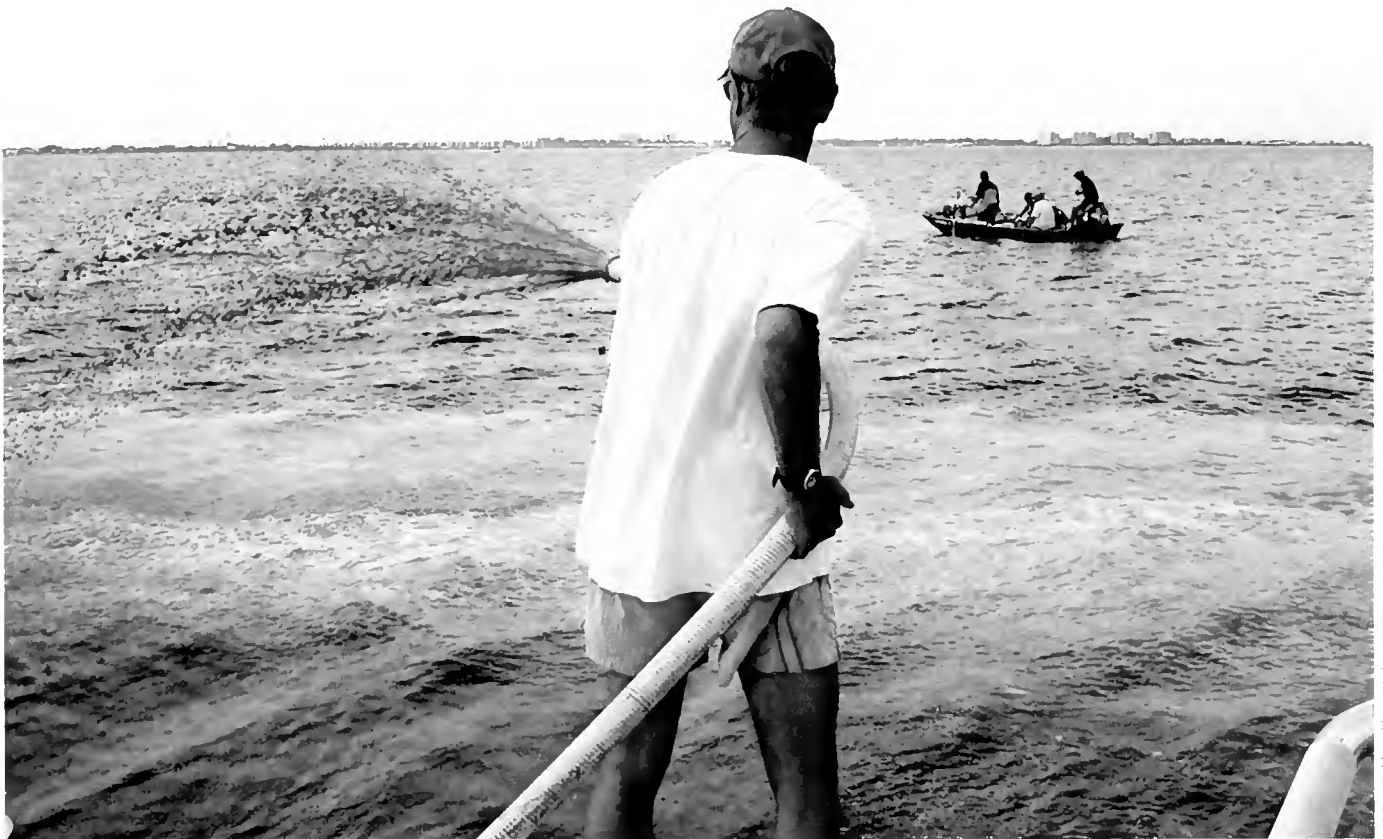
CLEANING UP WITH CLAY—Scientist Mike Henry of the Mote Marine Laboratory sprays clay slurries into Florida’s Sarasota Bay while WHOI Postdoctoral Investigator Mario Sengco and colleagues in the other boat track the dispersal of the plume with water sampling devices. The researchers are investigating the use of natural clays as a potential tool to mitigate harmful algal blooms, or “red tides.”
