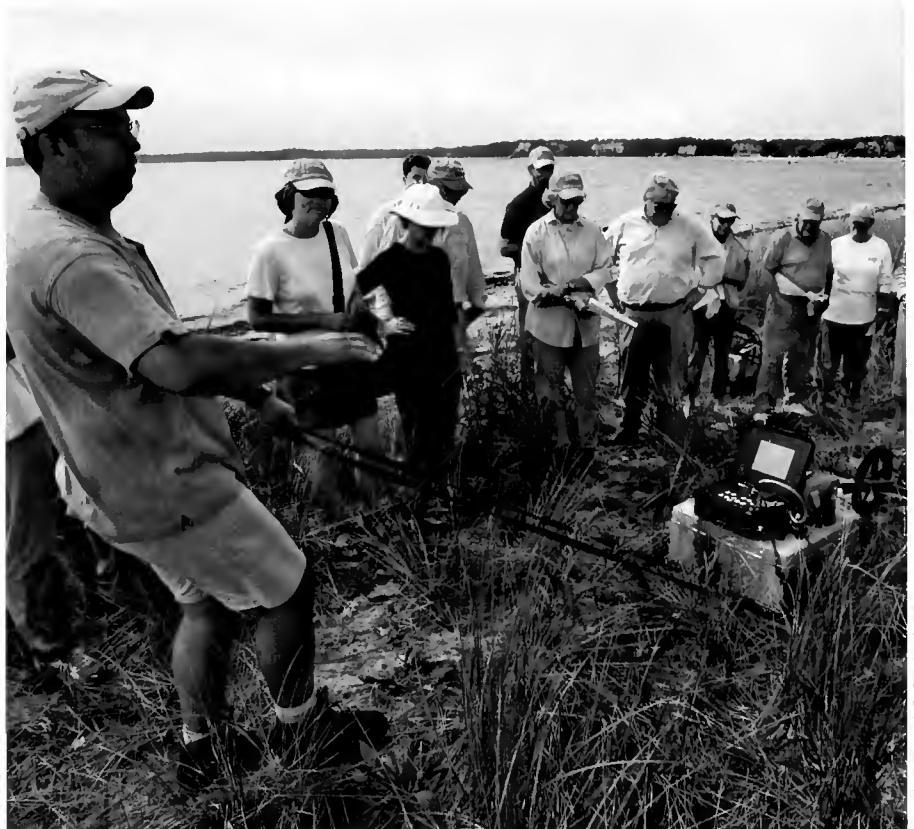
BURIED CLUES —WHOI Assistant Scientist Ilya Buynevich demonstrates a ground-penetrating radar instrument on a beach in Cotuit, Mass. By bouncing radar waves off buried rocks and sediments, he can create maps of subterranean layers and extrapolate past sea level.
