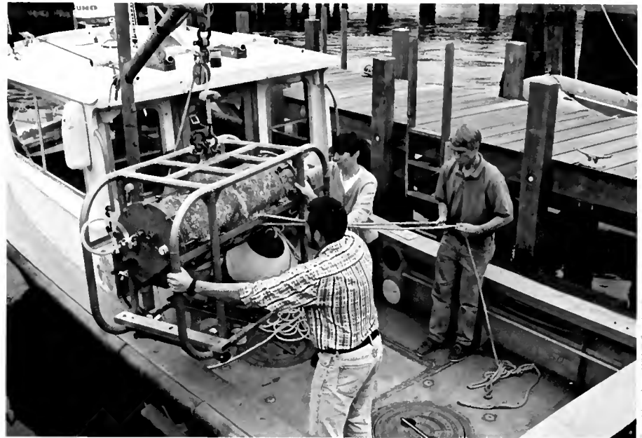
SHORE TO SHIP —WHOI researchers Alexi Shalapyonok, Heidi Sosik, and Robert Olson (left to right) carefully load the FlowCytobot onto a WHOI research vessel for installation on the seafloor at the Martha's Vineyard Coastal Observatory. The instrument counts and identifies protist cells in the water, and the data is transmitted via undersea cable back to shore.
