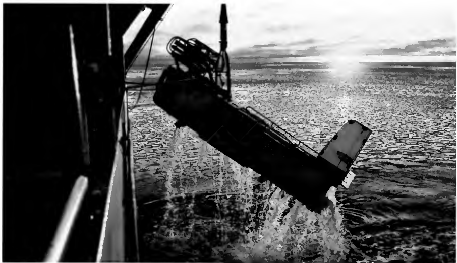
GOING FOR THE KRILL—BIOMAPER-II is lifted aboard the icebreaker Palmer, which cleared a path in the ice to tow the vehicle behind it. BIOMAPER-II has an acoustic system to detect plankton and zooplankton, a video plankton recorder to take pictures of them, and sensors to measure water properties.
