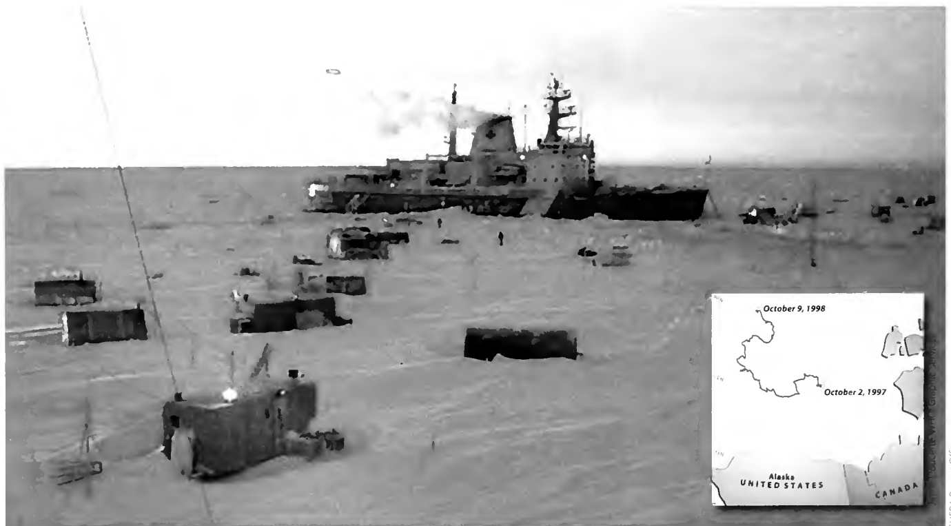
ICE CAMP—The Canadian icebreaker Des Groseilliers was purposely frozen into the Arctic ice for a year in 1997-98 to create a tiny, isolated camp with outlying laboratory structures. Inset: Drifting within the ice, the ship traveled more than 1,739 miles (2,800 kilometers) in a year.
