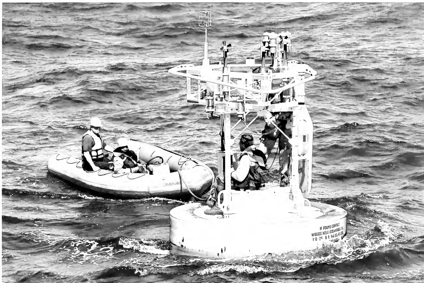
Members of the WHOI Upper Ocean Processes Group conduct at-sea repairs on an ASIMET buoy in the Gulf Stream that was probably damaged by a ship. ASIMET sensors measure heat, sunlight, winds, precipitation, humidity, barometric pressure, air and sea surface temperature, and salinity.
