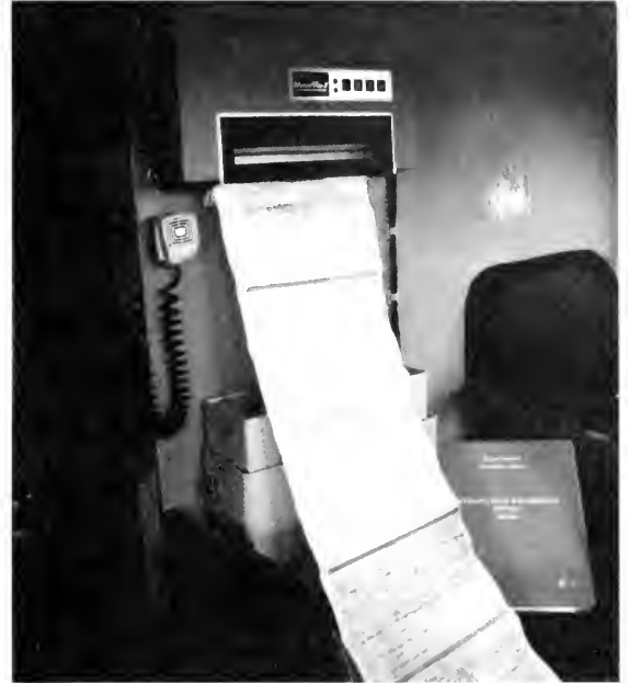
Figure 10. Radio-facsimile installations permit commercial fishing vessels to receive improved marine weather forecasts in chart form.
