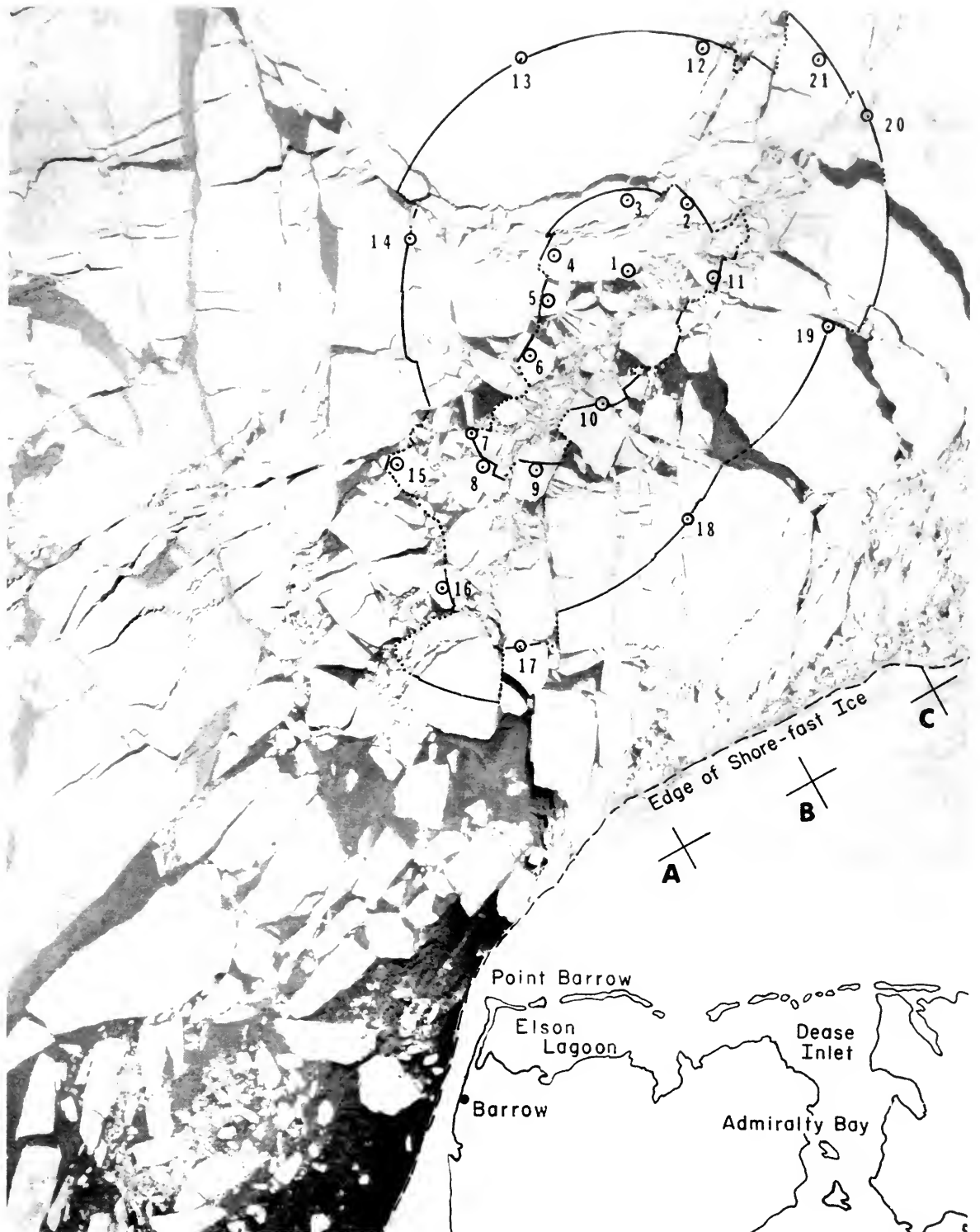
Figure 1. Landsat image (band 7) taken March 22, 1973, showing the deformation of the offshore pack near Barrow, Alaska. The indicated array of points was established three days earlier on two nested circles with diameters of 33 and 79 kilometers, respectively. Image width is 185 kilometers. (From Campbell, Weeks, Ramseier, and Gloersen, 1975)
