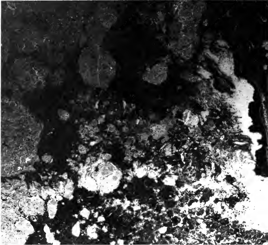
Figure 3. Seasat SAR image of sea ice on October 4, 1978, in the Beaufort Sea just west of Banks Island, N.W.T. Note the well-developed, large floes in the western part of the imagery. The image width is 100 kilometers. The dark areas are believed to be largely composed of flat, undeformed first-year sea ice. The uniform bright area running north-south in the eastern portion of the image is the result of sea clutter. (Courtesy Jet Propulsion Laboratory)
