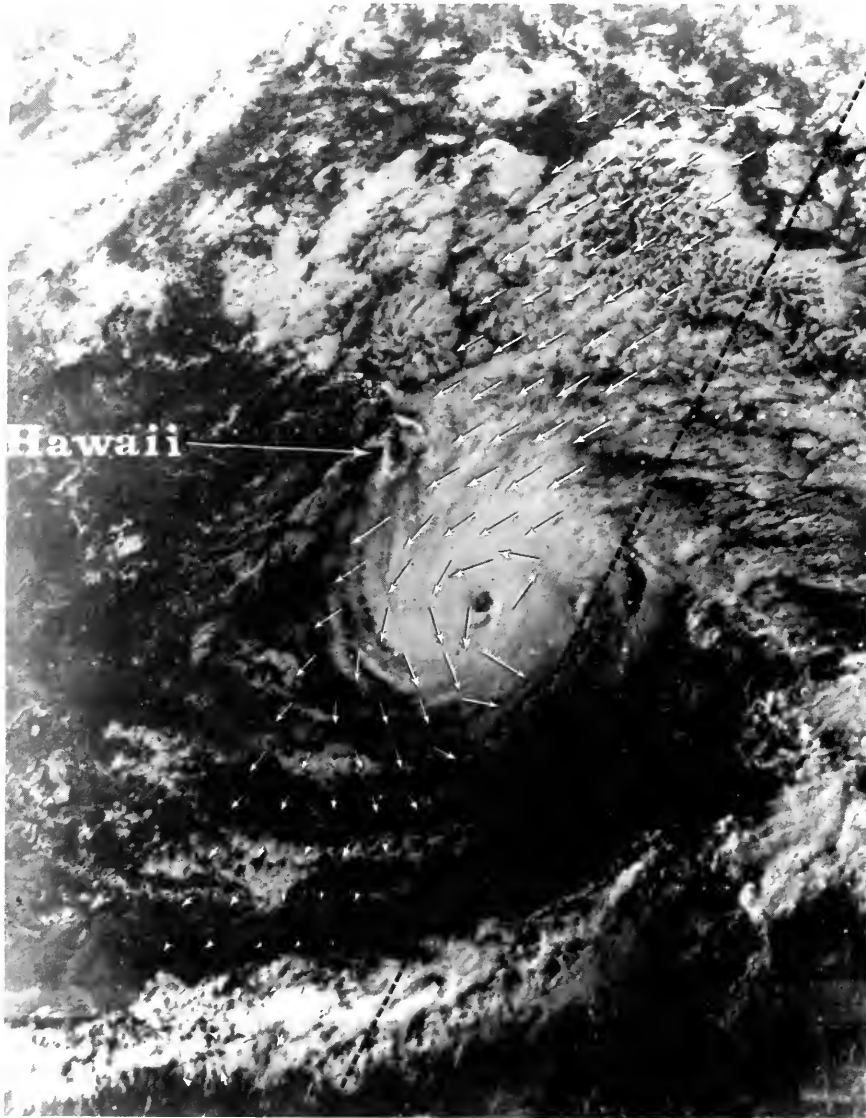
The ocean wind vectors of a hurricane. Data from the scatterometer wind measurement instrument aboard NASA's Seasat satellite determined, for the first time, the ocean wind vectors of a hurricane. The wind vectors (white arrows) sensed by the scatterometer are shown as an overlay on a NOAA satellite photograph of Hurricane Fico, taken just before Seasat flew over the hurricane on July 20, 1978. Seasat's sub-track is the black dotted line on the photo. (Photo courtesy of NASA)
