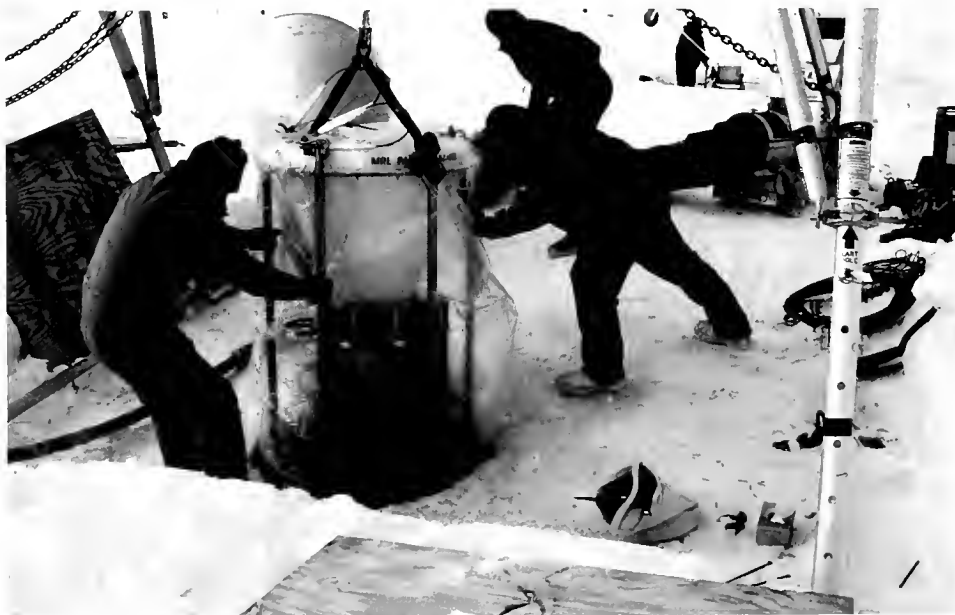
From left, John Kemp, Rick Krishfield, and Kiyoshi Hatakeyama deploy a time-series sediment trap through a hole they've drilled in the Arctic Ocean ice cover.
