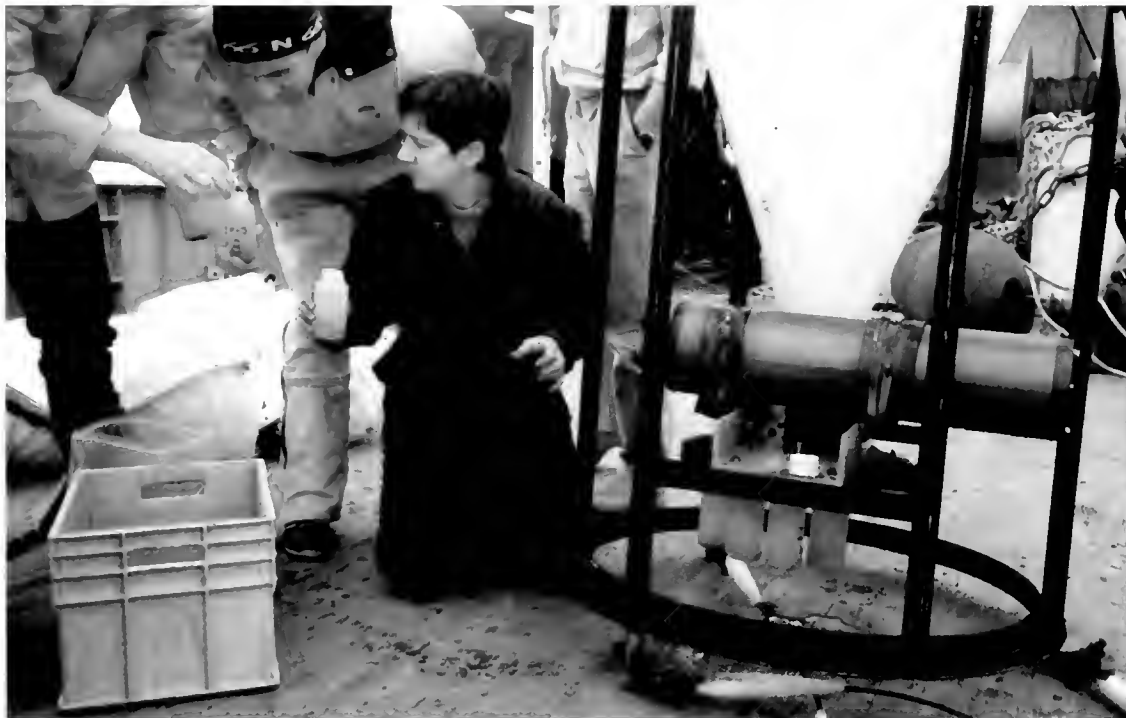
Research Associate Dorinda Ostermann removes sample cups from a sediment trap recovered aboard the Icelandic Research Vessel Bjarni Saemundsson .
