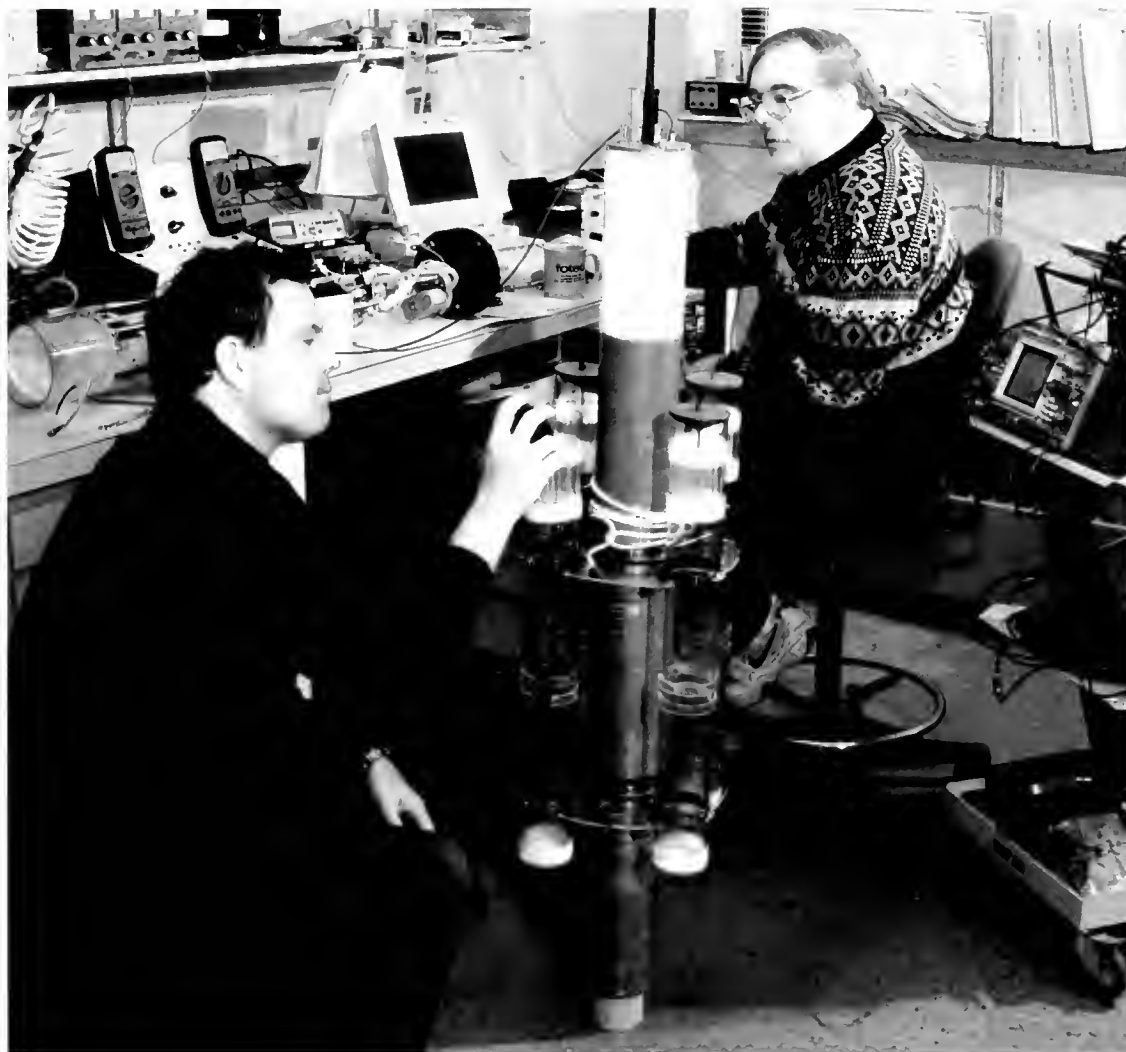
Jim Price (left) and Jim Valdes with a prototype of the neutrally buoyant sediment trap. The four small plastic tubes collect sediment and the large central tube houses electronics, a variable displacement device, recovery beacons, and batteries.
