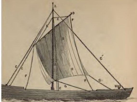
Fig. 1. RIGGING OF HOMERIC SHIP.
