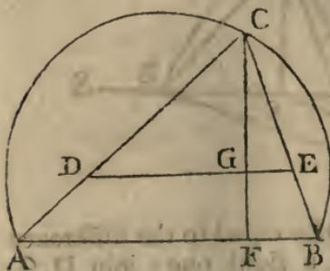
Take  $AF$  to  $FB$  in the given ratio of the segments of the base, and upon the right-line  $AB$  describe a segment of a circle  $ACB$  capable of the given angle; make  $FC$  perpendicular to  $AB$  meeting the circumference of the circle in  $C$ , in which
