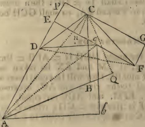
Make a right-angle  $b$  with two of the given lines  $Ab, bc$ ; and with the other two complete the trapezium  $AbcD$ : upon  $AD$  let fall the perpendicular  $cE$ , in which produced (if necessary) take  $EF$ , so that the rectangle
