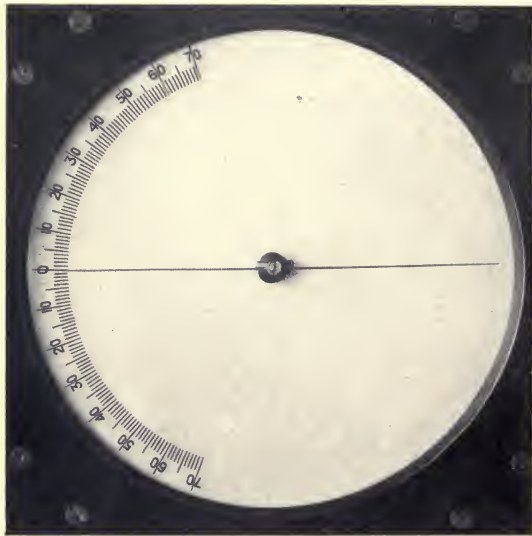
DIAL OF INSTRUMENT SHOWING NEEDLE WHICH IS DEFLECTED BY THE HIDDEN OIL.
