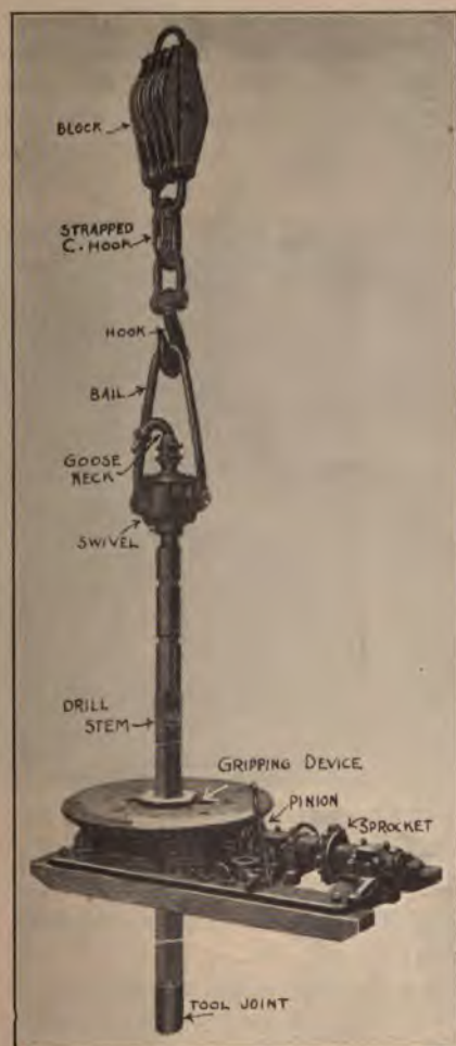
FIG. 18.—Rotary-drilling outfit. Shows driving and gripping devices.
