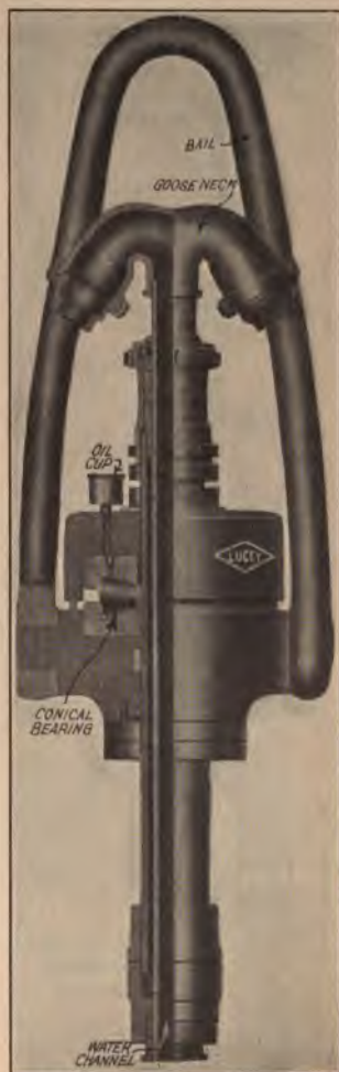
FIG. 20.—Swivel for rotary drilling.
