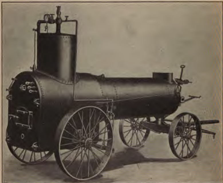
FIG. 25.—Twenty to 25 h.p. oil country boiler. Locomotive type. (Internally fired.)
