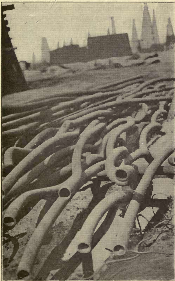
FIG. 52.—Tubing fished from a well, after having dropped several hundred feet.
