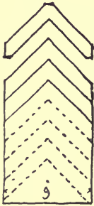
FIGS. 60, 61. METHOD OF FORMING RIDGE CRESTING.
