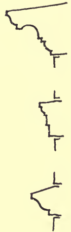
FIG. 56. TYPICAL PROFILES OF CHIMNEY CORNICES.
