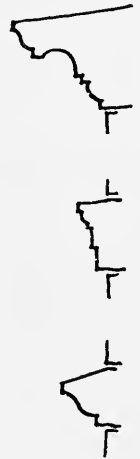
FIG. 56. TYPICAL PROFILES OF CHIMNEY CORNICES.
