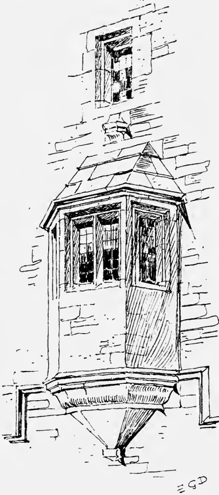
FIG. 83. ORIEL WINDOW AT BURFORD.
