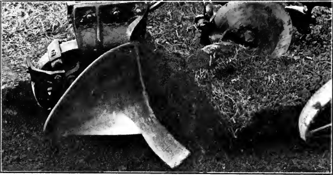
A section of the furrow shown in the illustration on page 116 cut farther forward, showing that the plow bottom has forced the furrow slice to conform to its shape, thereby beginning a stretching operation on the bottom of the furrow. Observe in the illustration on page 116 that after the furrow slice has reached the ground the freshly stretched furrow slice bottom is helping to put pressure against the top.
