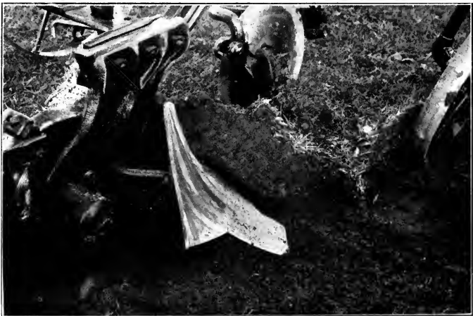
A plow bottom which does not have the proper shape to force the furrow slice against its surface so that the pressure is equal on all parts of the plow bottom. This illustration shows the importance of having a plow bottom adapted to the soil. The shin is doing the greater part of the work.
