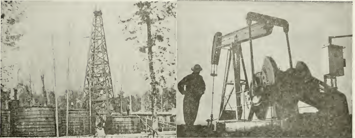
The picture at left is of an early oil well. At right, the modern petroleum engineer employs the principle of the simple suction pump to lift oil to the surface.
