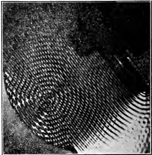
FIG. 350.—Instantaneous photograph of waves on the surface of mercury. (By J. H. Vincent.)
