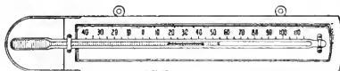
FIG. 270.—A minimum thermometer (as used in the Meteorological Service). It is hung in a horizontal position.
