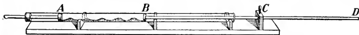
FIG. 206.—The little heaps of powder in the tube are produced by the vibrations of the disc B .
