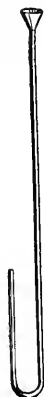
FIG. 138.— Air compressed within a closed tube by weight of mercury in the long branch.
