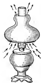
FIG. 316.—Air currents produced by placing a jacket around a heated body.
