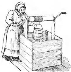
Fig. 89.—Windlass used in drawing water from a well.
