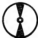
FIG. 407.—Disc to put over Newton's disc to cut out any desired colour.
