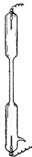
FIG. 420.—A tube for holding a gas to be examined by the spectroscope.
