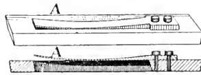
FIG. 245.—An organ reed. The tongue A moves in and out of the opening. This is called a free reed.
