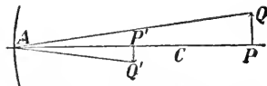
FIG. 356.—The size of the object PQ is to that of the image P'Q' as their distances from the mirror.
