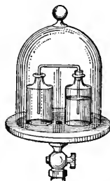
FIG. 140.—Water forced out of the closed bottle by the expansion of the air above it.
