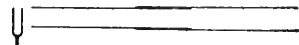
FIG. 225.—The length of an open tube when in resonance with a tuning-fork is one-half the wave-length of the sound.
