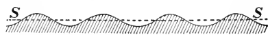
FIG. 190.—Small waves, or ripples, on a liquid, due chiefly to surface tension.
