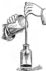
FIG. 185.—How to utilize surface tension in pouring a liquid.
