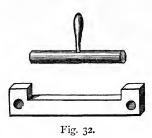
also accurately into this gauge; but if I make it warm with this spirit-lamp, it will only go in the gauge or through the hole with difficulty; and if I were to put it into boiling-water, it would not go through at all. Again, as soon as the
