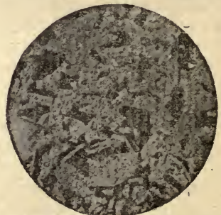
FIG. 17.—SAME STEEL HEATED TO 1,200° CENT. (2,192° FAHR.) AND COOLED SLOWLY IN THE FOUNDRY
