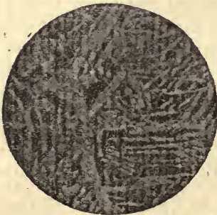
FIG. 16.—SPECIMEN OF CAST STEEL IN CONDITION AS CAST (AIR COOLED)
