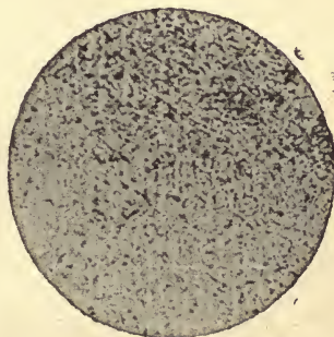
FIG. 19.—SAME STEEL HEATED TO 800° CENT. (1,472° FAHR.) AND COOLED IN AIR. AN IDEAL STRUCTURE FOR STEEL CASTINGS
