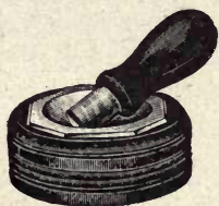
FIG. 10.—Agate mortar and pestle for finely pulverizing coal.
