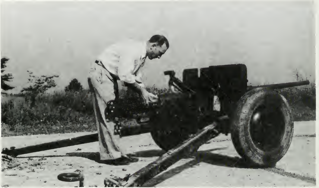
LABORATORY FOREMAN LOADING 37-MM. ANTITANK GUN for test shot at Erie Proving Ground, July 1941.
