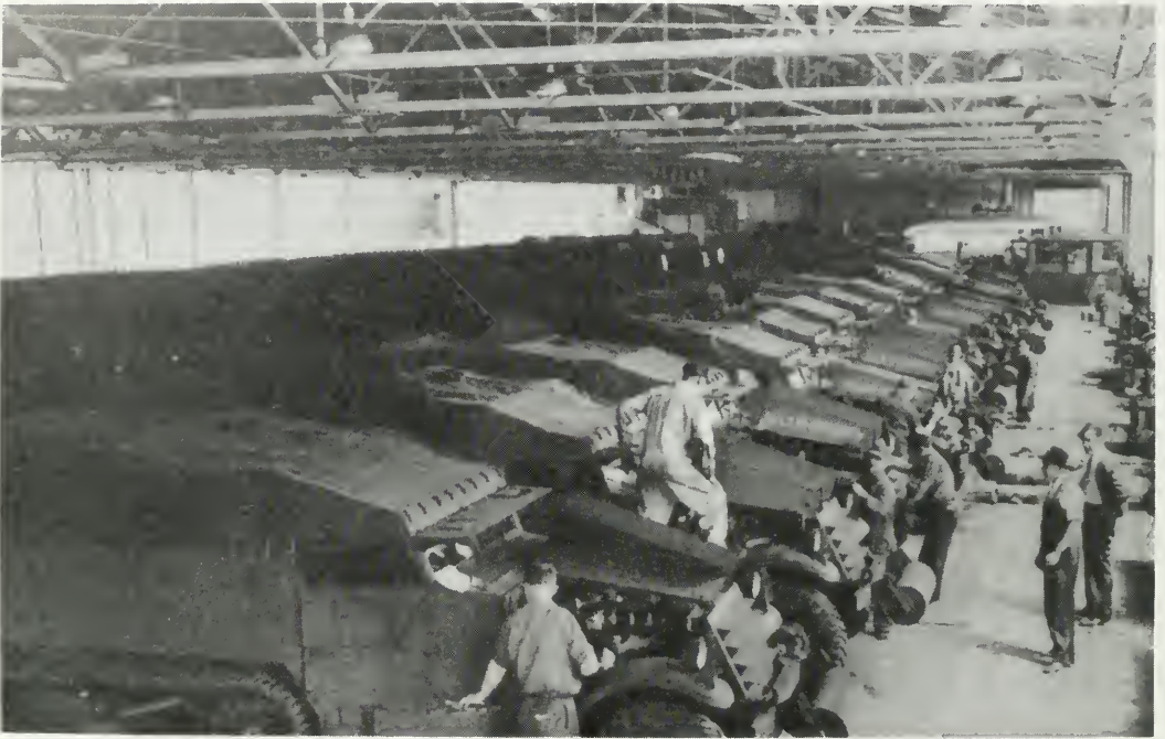
HALF-TRACK CARS M2, built primarily to transport cargo and personnel in combat areas, nearing completion at the White Motor Company, June 1941.
