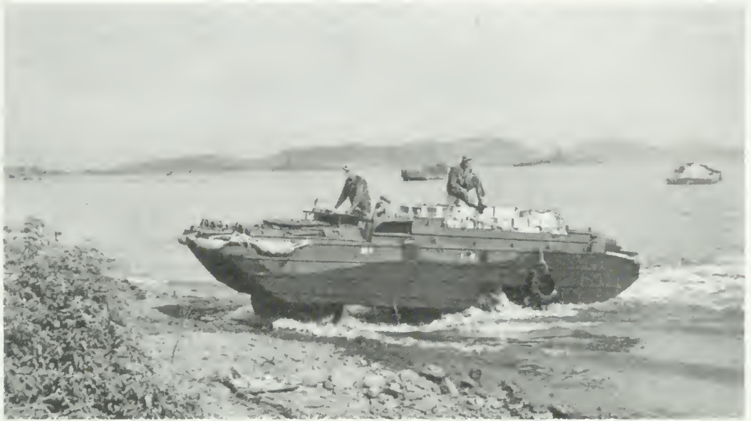
DUKW, 2½-TON AMPHIBIAN TRUCK, leaving the water with cargo, Noumea, New Caledonia, April 1943.
