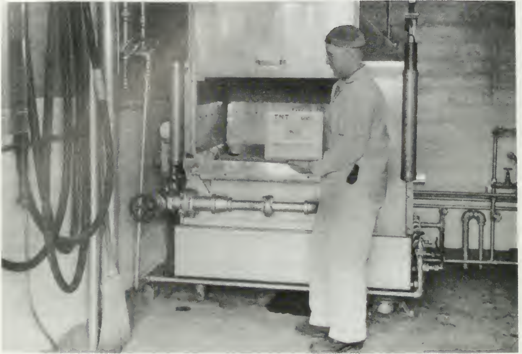
BOX OF BULK TNT being processed in the melt unit is handled by a workman wearing nonsparking safety shoes made without nails.
