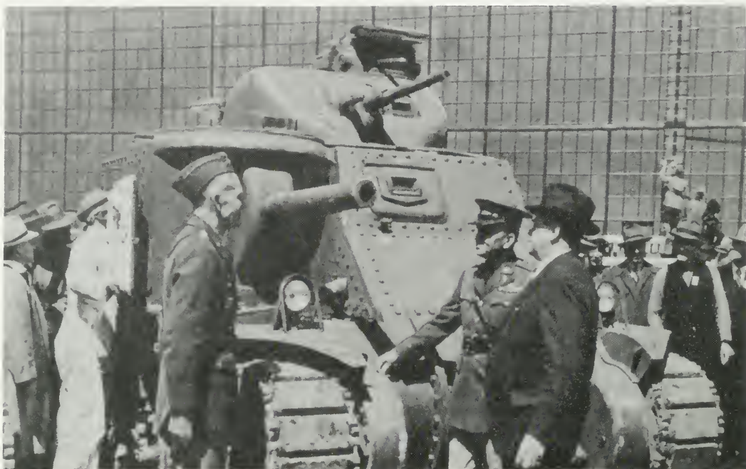
M3 MEDIUM TANK MOUNTING A 75-MM. GUN delivered to the U.S. Army by the Chrysler Corporation. Standing in front of the tank from left: Brig. Gen. Adna R. Chaffee, Maj. Gen. Charles M. Wesson, and Mr. K. T. Keller.
