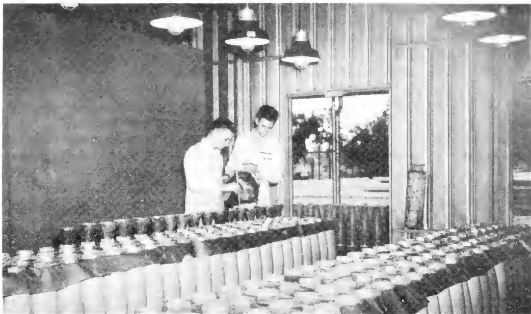
WORKMEN POURING MOLTEN TNT INTO 155-MM. SHELLS at Charleston Ordnance Depot, October 1941.
