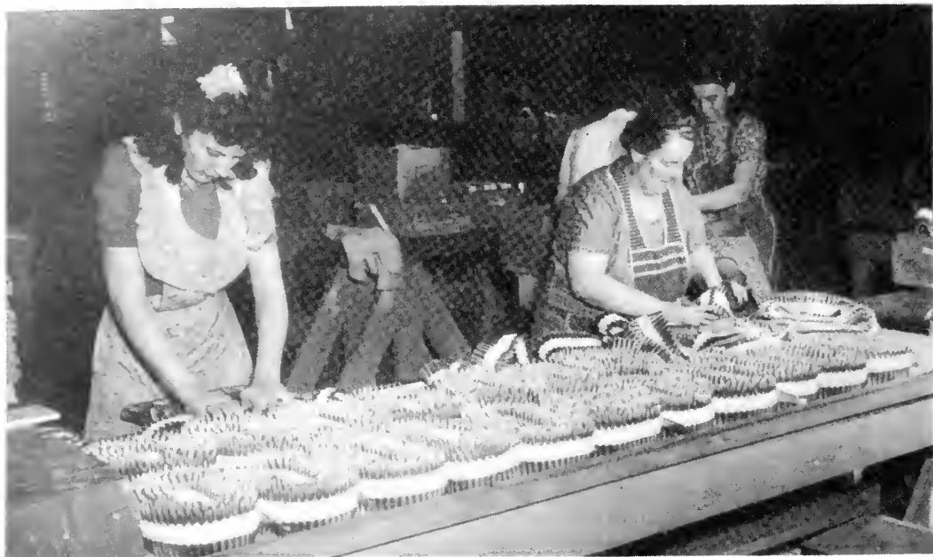
.50-CALIBER MACHINE GUN AMMUNITION IN FABRIC BELTS, being arranged for crating by women in an ordnance arsenal.
