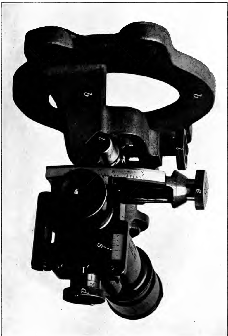
Fig. 240.—Telescopic Sight, Model 1898.
