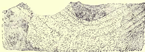
FIG. 22.—Section of the northern end of the Cherry Valley Mine. 1, Clay detritus; 2, Sandstone; 3, Cherty and slaty clay; 4, Ores; 5, Blocks of sandstone. After F. L. Nason, Report on Iron Ores of Missouri, p. 131.
