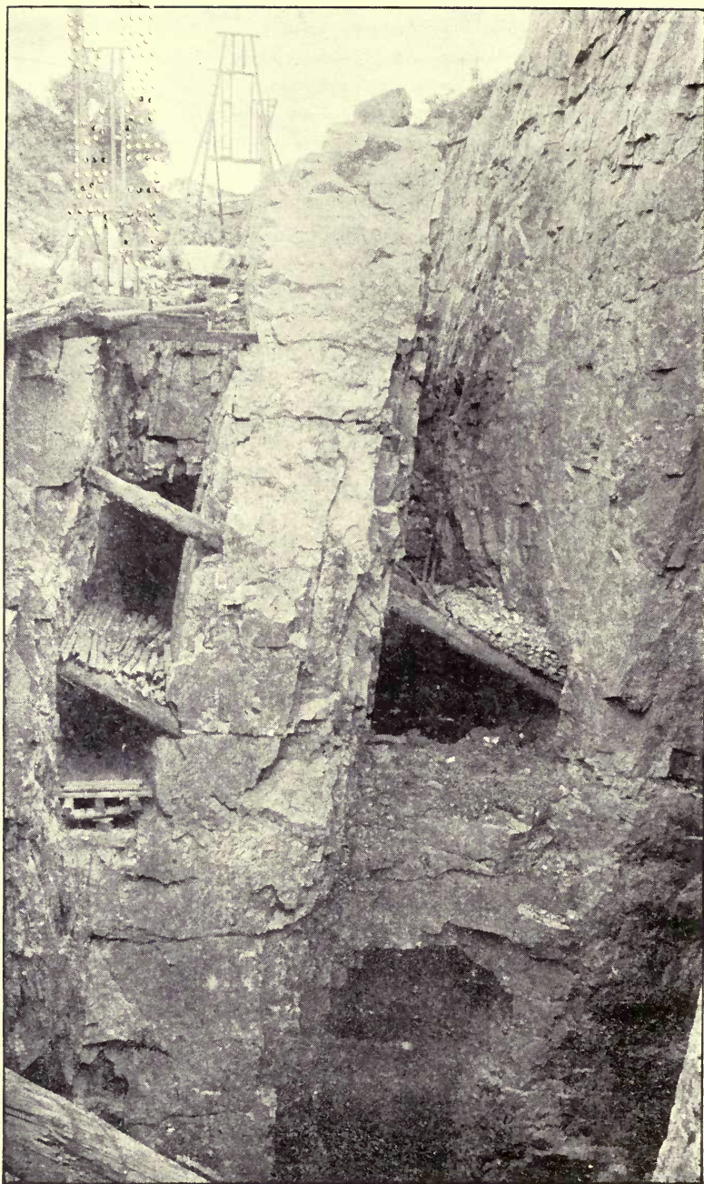
FIG. 29.—Open cut in the Republic mine, Marquette range, showing a horse of jasper. From a photograph by H. A. Wheeler.
