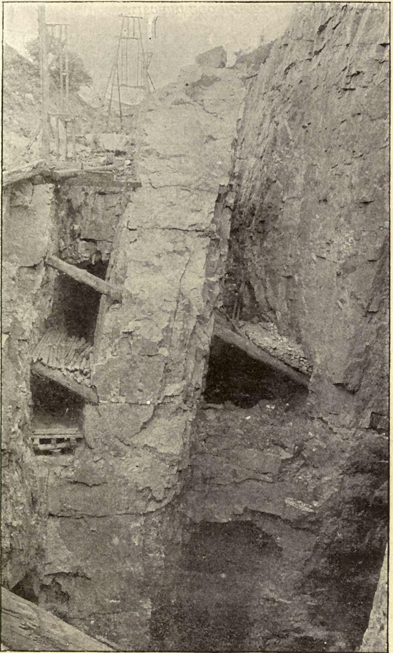
FIG. 17.—Open cut in the Republic mine, Marquette range, showing a horse of jasper. From a photograph by H. A. Wheeler.
