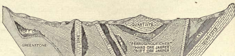
FIG. 1.—GENERALIZED VERTICAL SECTION IN MARQUETTE DISTRICT, MICHIGAN, SHOWING RELATION OF DIFFERENT CLASSES OF ORE-DEPOSITS TO ASSOCIATED FORMATIONS.
