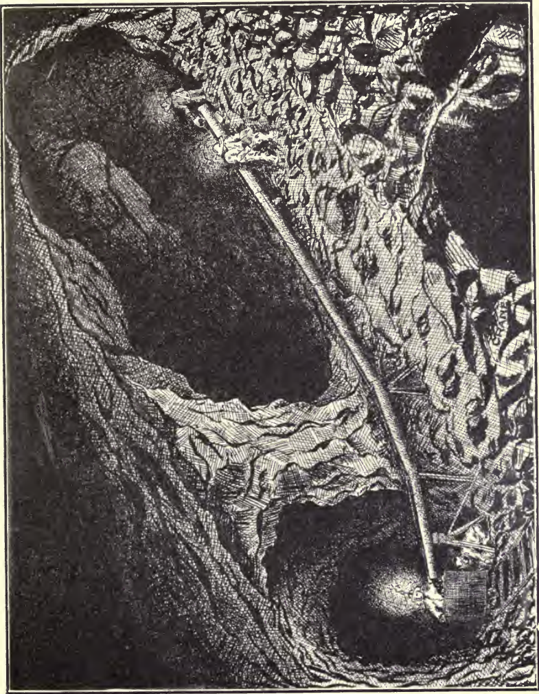
FIG. 20.— Loading Cars by Chute, Mohawk Mine.
