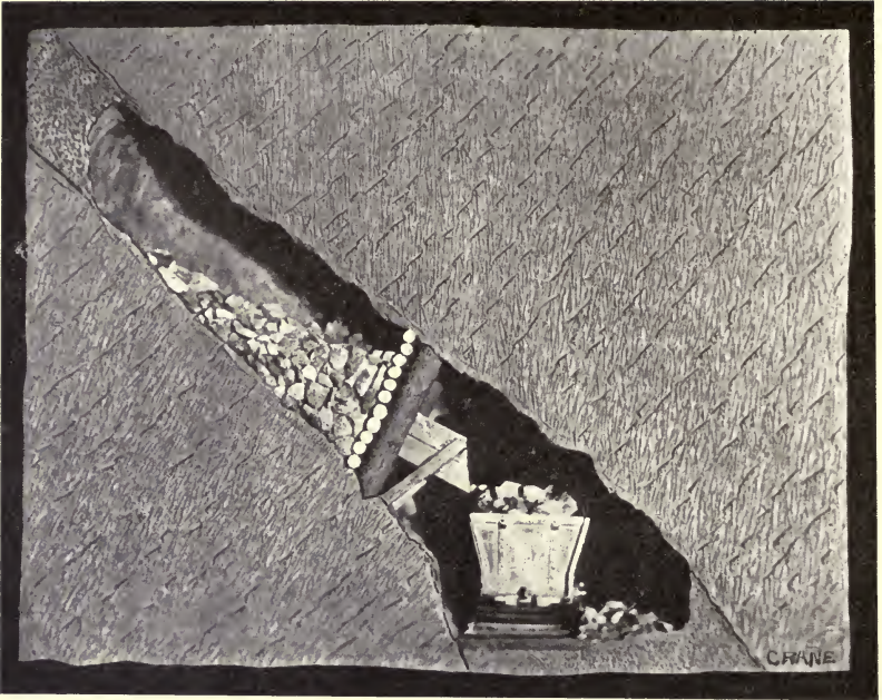
FIG. 2. — Position and Use of Stull in Vein.
