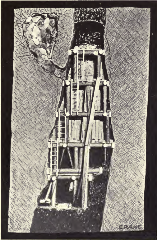
FIG. 34. — Vertical Section through Vein Showing Method of Placing Stull-Sets. (Modeled after Sketch by Robert N. Bell.)
