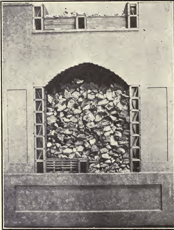
FIG. 60. — End View of Stope in Homestake Mine, Back-Filling Method. (From Model in Engineering Office of Company.)
