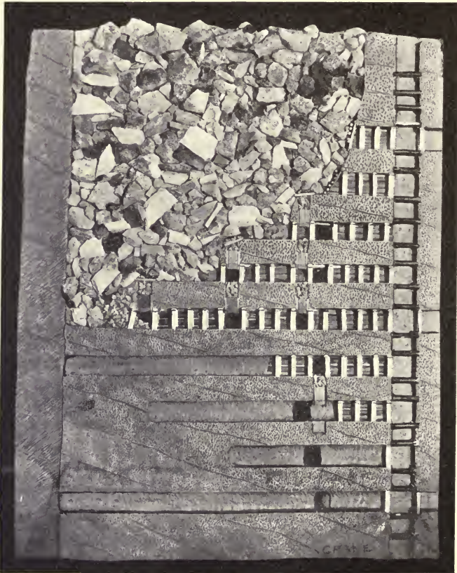
FIG. 45.—Longitudinal Section through the Sub-drifts Showing the Incline on the Right, also Other Passages Driven across the Deposit from the Sub-drifts.
