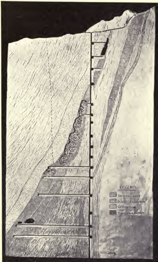
FIG. 9. — Vertical Section through Shaft and Orebodies of the Alaska-Treadwell Mines. (Modeled after Sketch in Mining and Scientific Press, Feb. 10, 1917.)
