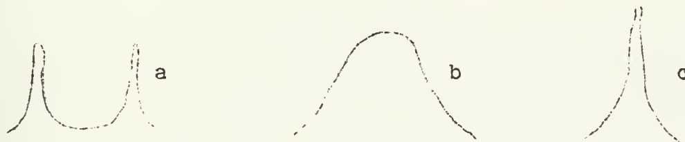
Figure 2. NMR Spectra for conformational isomers with a) slow, b) intermediate and c) rapid internal rotation. Intensities are not to scale.
