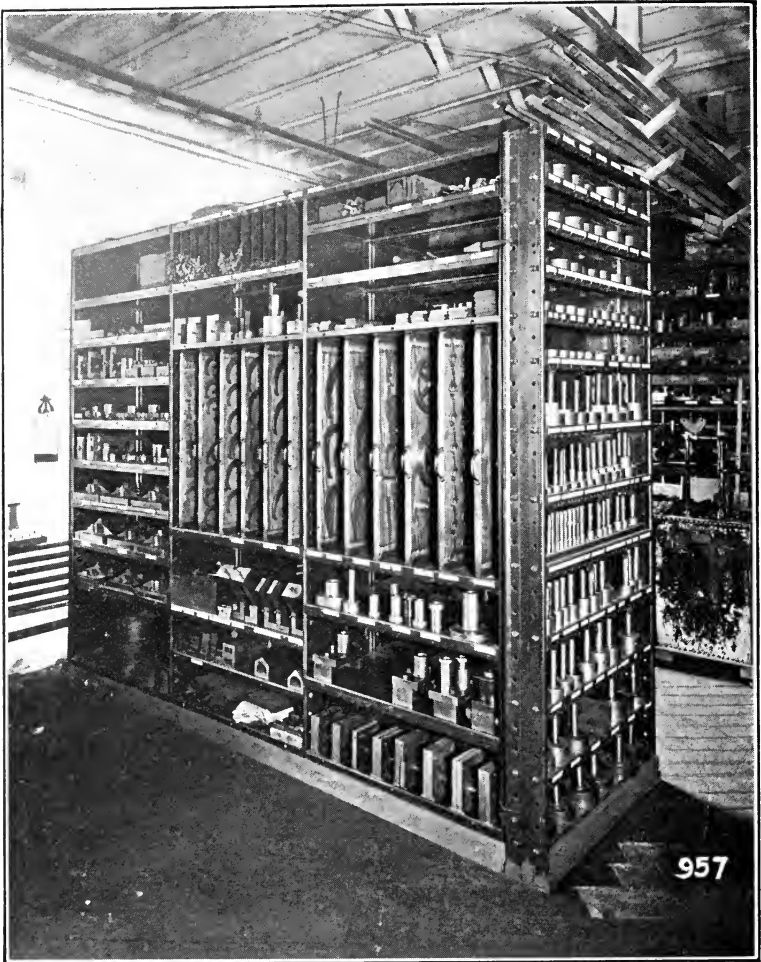
FIG. 117.—Tool Room Section made up of Standard Shelving with sliding panels for snap gauges, lathe dogs, milling cutters and similar equipment. Panels are equipped with hooks and with label giving the number of the various tools. Check hooks are provided for carrying the workman's check. These sliding panels give a much more compact arrangement for carrying snap gauges, milling cutters, and the like, than the usual method of hanging these on boards along the wall. Another feature of this rack is the special section for plug gauges as shown at the end of the rack.
