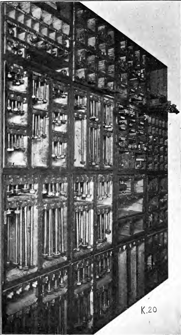
FIG. 115.—Tool-room section made up of tiers of racks, and each compartment subdivided with boxes labeled with brass plates, giving the size and symbol of the bolts contained therein. Particular attention is called to the method of stocking the bolts; the sizes and lengths of the bolts regulate the sizes of the boxes. Pegs are provided on the front of the bottom beveled edge for the workman's checks.
