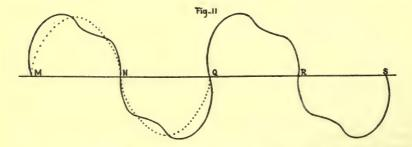
The resultant curve shows the influence of additional overtones and may be used to represent the vibrations of the tone of a Salicional pipe.
