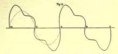
result of such a combination is indicated. As in all the illustrations, the dotted line indicates the curve of the fundamental vibration of the tuning fork. In this resultant curve, the absence of the influence of the first overtone is pronounced.
