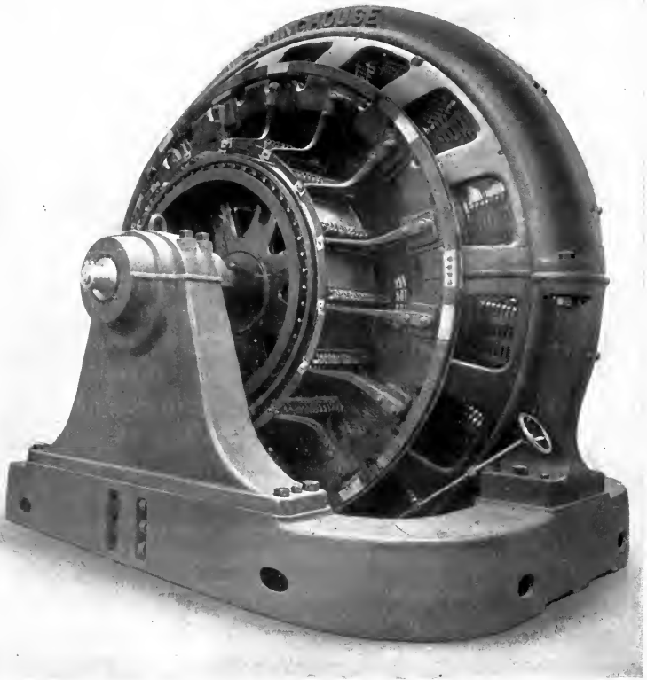
FIG. 23.—3,000 K.W., 600 Volt, 25 Cycle Rotary Converter.
