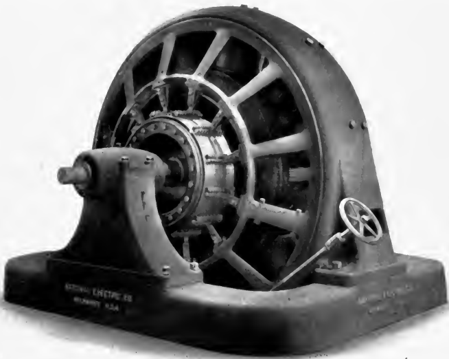
FIG. 18.—1,000 K.W. 600 Volt, 25 Cycle Rotary Converter.
