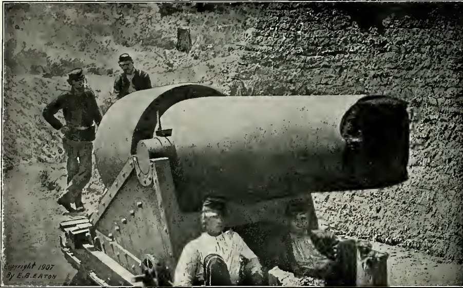
300-POUNDER PARROTT GUN IN BATTERY STRONG AFTER BURSTING OF MUZZLE
