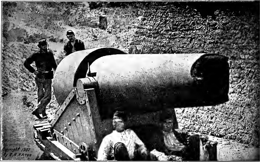
300-POUNDER PARROTT GUN IN BATTERY STRONG AFTER BURSTING OF MUZZLE
