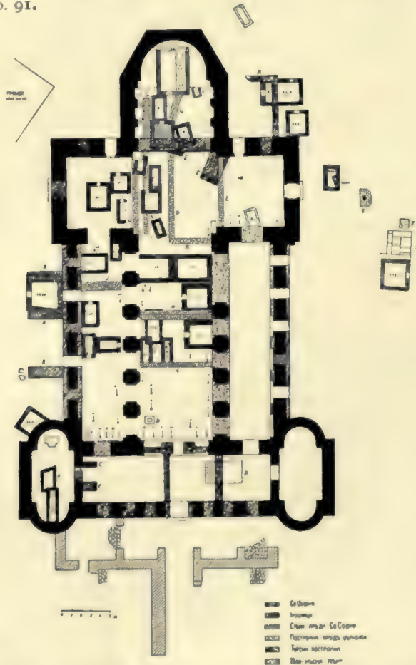
20 Sofia, Church of S. Sophia, cruciform domed church with three aisles ; plan ; after Filow. See p. 91.
