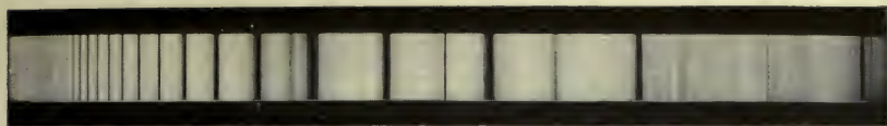
FIG. 17. Spectrum of Zeta Tauri from H_{\gamma} to limit of Balmer series (last line showing H_{31} ) made with 37\frac{1}{2} inch reflector. These hydrogen lines are all absorption lines, reversed against the continuous background of the stellar emission spectrum.
