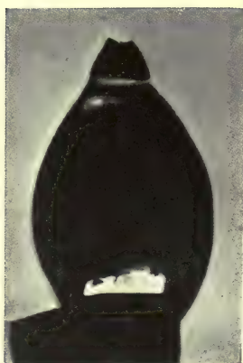
FIG. 15A. Illustrating the practically complete absorption of rare mercury vapor for the resonance radiation \lambda 2537.
